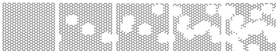
Fig. 1 Simulation box with graphene layers at the bottom. The outermost graphene layer is made defective with a defect percentage and a defect radius
